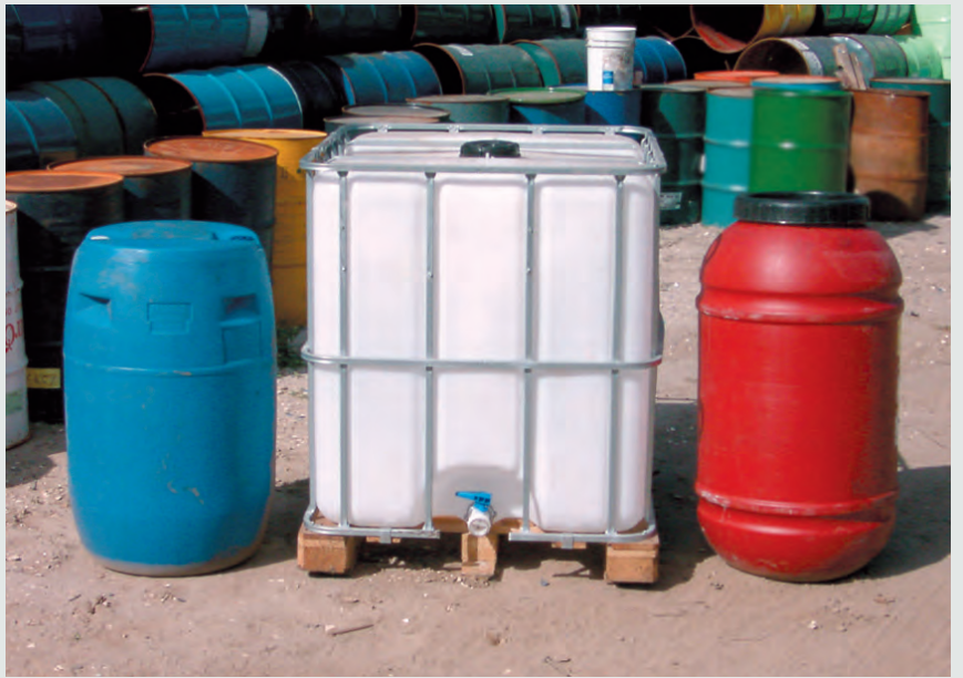
Some common containers used for rain barrels are (left to right): 50-gallon sealed barrel, 275-gallon IBC tote (juice container), and 50-gallon open top barrel.
