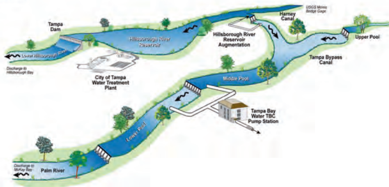
A schematic of the Hillsborough River and the Tampa Bypass Canal showing the City of Tampa's and Tampa Bay Water's withdrawal points.
