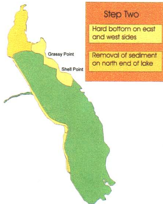
Figure 1. Step Two - Dredge to Hard Bottom from 35' Contour - entails dredging on east side of lake in vicinity of Shell and Grassy Points, along most of western shoreline. Although sediment deposits are deep, the north end is dredged to prevent material from this area being transported into hard bottom areas.
